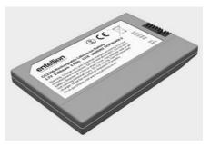
When being discharged in the host device, the traditional battery cannot provide any form of run time prediction and host devices must resort to crude voltage measurements to provide an approximation of remaining capacity. Such systems become unreliable with changes in temperature and are also affected by battery ageing due to an increase in resistance, resulting in a reduction in the voltage under load.
