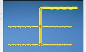
The Distribution and Feeder configuration is the basic, economic layout used to route cables out of the MDA. A higher capacity Distribution Run is used to supply the feeders that route cables out to the cabinets in the EDA. The Feeders in turn are positioned over the cabinet line ups to create a pathway that will provide efficient transitions to the vertical cable management areas of the cabinets and not interfere with Cold Aisle cooling air flow.
